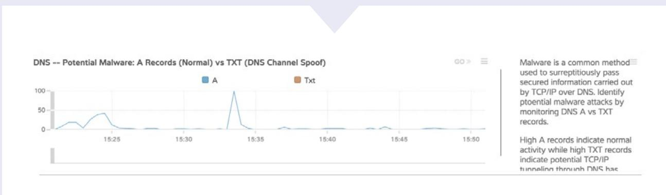
DNS-TXT request may indicate an attempt to tunnel protocols (e.g. SSH, HTTPS) via DNS. The affected device then recorded an increased volume of DNS TXT queries.
